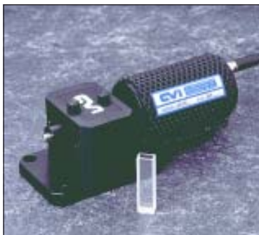
AT-SHC Fiber Optic Sample Holder (shown with ASB-W-003 light source)
