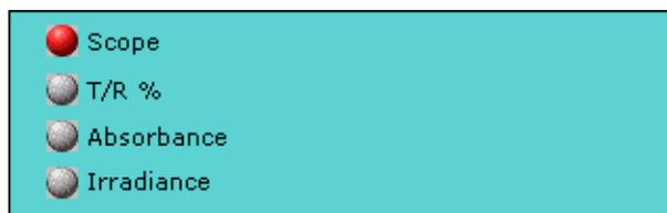
If irradiance is chosen, the irradiance options for absolute or relative measurements and the distance will appear to the right of the selections. There are two kinds of irradiance measurements. The Absolute Irradiance needs to be calibrated by using a calibrated light source. Distance, is the distance from the light source to the unit, and Relative Irradiance needs the calibrations spectrum of the light source, and the color temperature of the light source.
