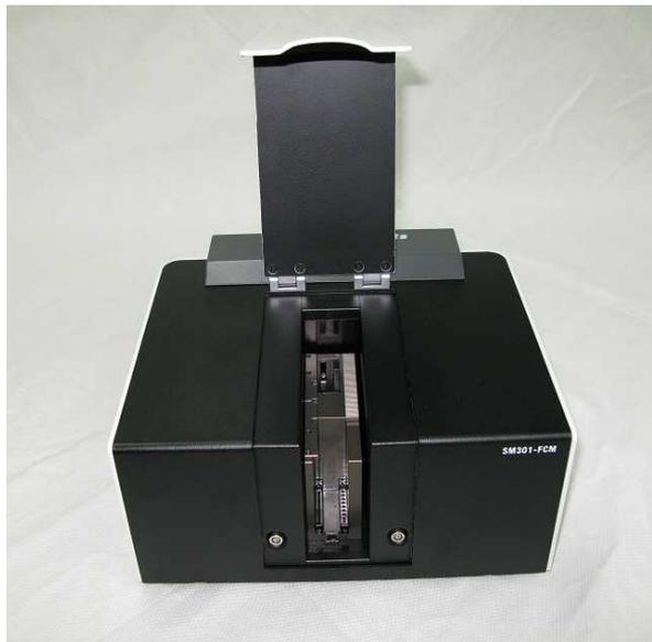
3. Place the reference (empty) cuvette in the “REF” slot.
