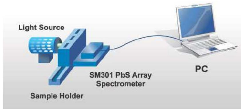
The PbS array spectrometer is based on a crossed Czerny-Turner configuration and consists of an entrance slit, a gold coated collimating mirror, a grating, a gold coated focusing mirror a gold coated bending mirror, and 256 pixels PbS array detector.
