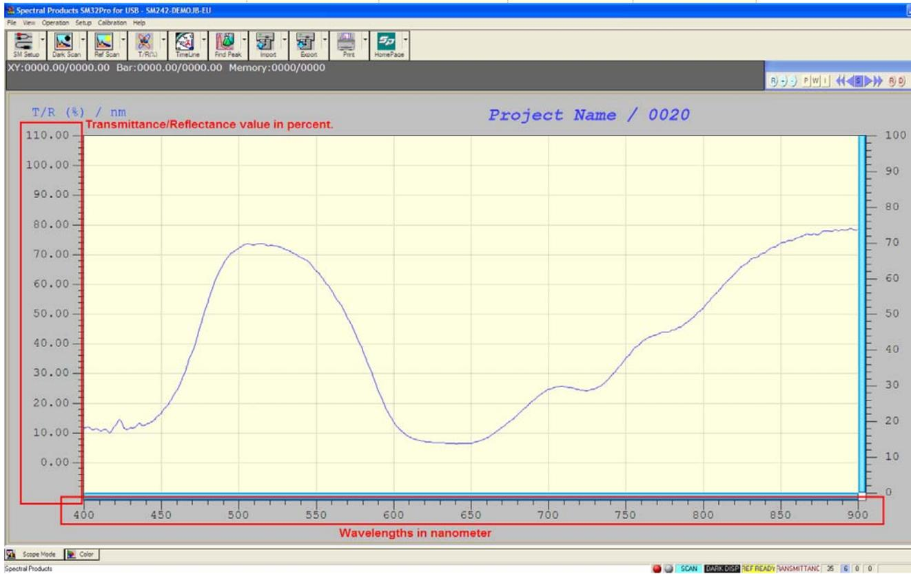
First, you need to change the display mode to “T/R %” mode to see the Transmittance or Reflectance in percent (%). Click the black arrow next to the “Scope” toolbar button (#1). It
