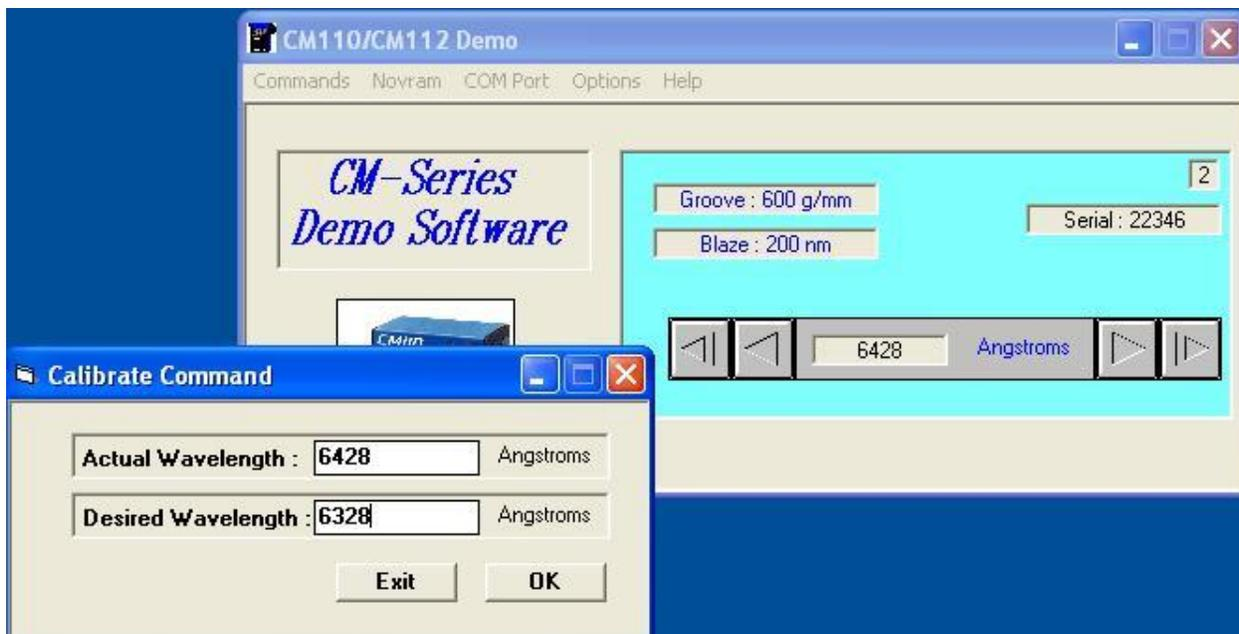
In the above example, from our known wavelength of 0nm, and after issuing a GoTo 632.8nm, we had to step the grating up to 642.8nm to get the laser light to exit. Entering 632.8nm into the **Desired Wavelength** box and clicking **OK** will make the Warning box appear. Clicking **Continue** will calibrate the grating:
