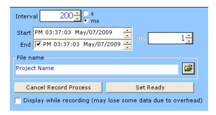
The **Timeline** button will become **Ready** after all timeline recording parameters are set. Click on the "**Set Ready**" button to start the timed recording process to record spectra within the set duration as shown in the timeline dialog box. The "Cancel Record Process" will cancel the process.
