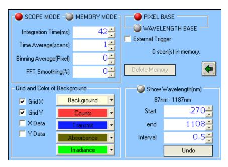
**SCOPE MODE** is the default-operating mode, which enables the live updating of data acquisition.
