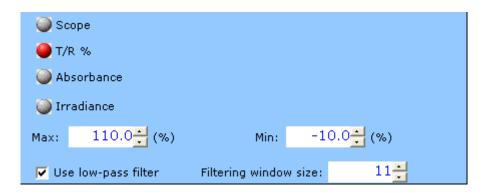
The "Scope" mode shows the signals read by each CCD pixel in 16-bit scale.
