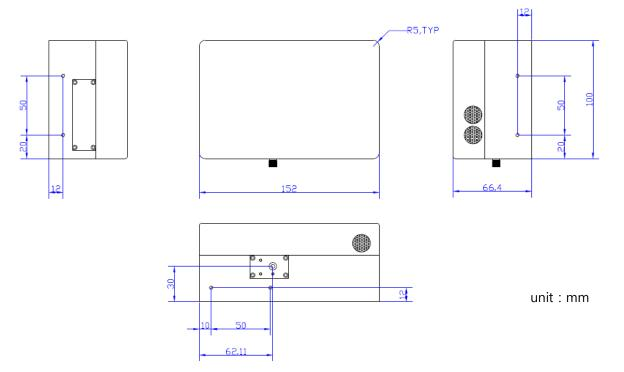
Ordering Information : Please indicate product number plus description when ordering SM642N Low Noise Non-TE-Cooled Back-thinned CCD Ethernet Communication Spectrometer
