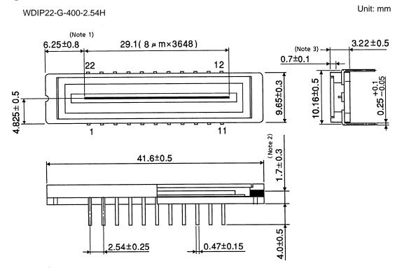
Note 1: Distance between the edge of the package and the first pixel (S1) Note 2: Distance between the top of chip and bottom of the package Note 3: Glass thickness (n = 1.5)
